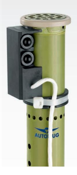
The AUTOFLUG Optical Fuel Level Sensor (OFLS) is a small sensor for installation inside fuel tanks. The sensor is designed for dedicated point level sensing (e.g. low or high level sensing) as well as for control of fuel transfer, refuelling and defuelling functions. Typical applications are helicopter and fixed wing aircraft fuel tanks.
