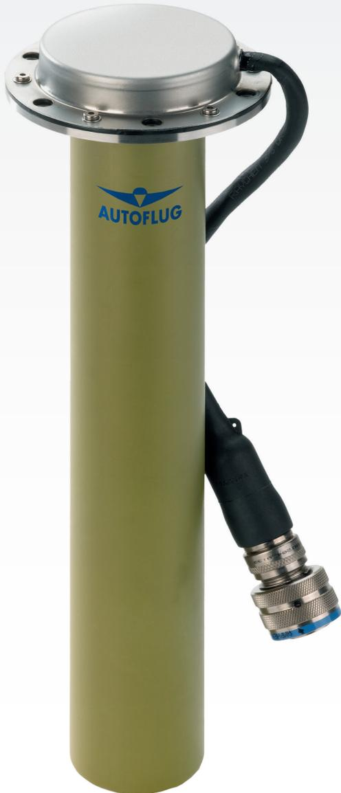
The AUTOFLUG CAN Bus compatible capacitance type Fuel Gauge Transmitter (FGT) provides temperature compensated fuel quantity measurement. The sensor provides highly accurate fuel contents information in litre, kg, lbs, etc. over the complete temperature range of a specific fuel type. The fuel gauging length can be adapted in accordance with customer requirements.
