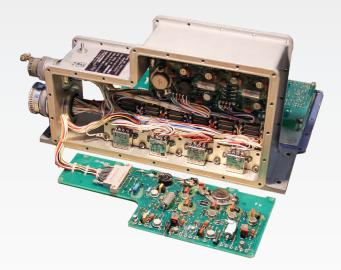
The control unit decides electrically as to whether the thermistor body is immersed in the fuel or is situated in air and/or fuel vapors. Dry thermistor bodies will cause a smaller drop in voltage and wet thermistor bodies will cause a larger drop in voltage. This characteristic is used in order to activate and/or deactivate relays.
