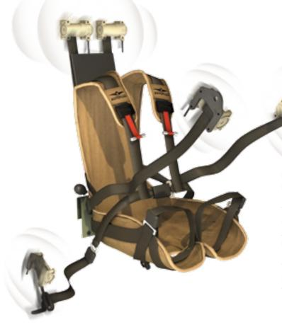
The safety seats and other cabin fixtures use a unique textile damping system which isolates the vehicle structure using textile components. This makes our products lightweight and robust, ensuring high flexibility in narrow and often tight vehicle cabins.
