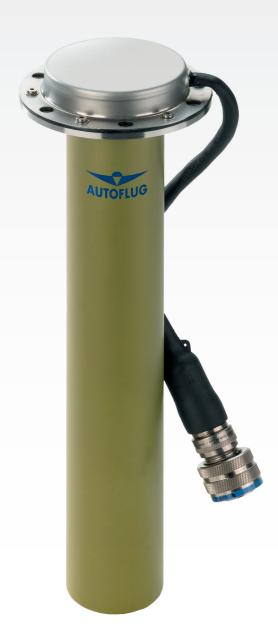
The AUTOFLUG CAN Bus compatible capacitance type Fuel Gauge Transmitter (FGT) provides temperature compensated fuel quantity measurement. The sensor provides highly accurate fuel contents information in litre, kg, lbs, etc. over the complete temperature range of a specific fuel type.
