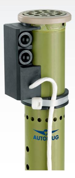
The AUTOFLUG Optical Fuel Level Sensor (OFLS) is a small sensor for installation inside fuel tanks. The sensor is designed for dedicated point level sensing (e.g. low or high level sensing) as well as for control of fuel transfer, refuelling and defuelling functions. Typical applications are helicopter and fixed wing aircraft fuel tanks.
