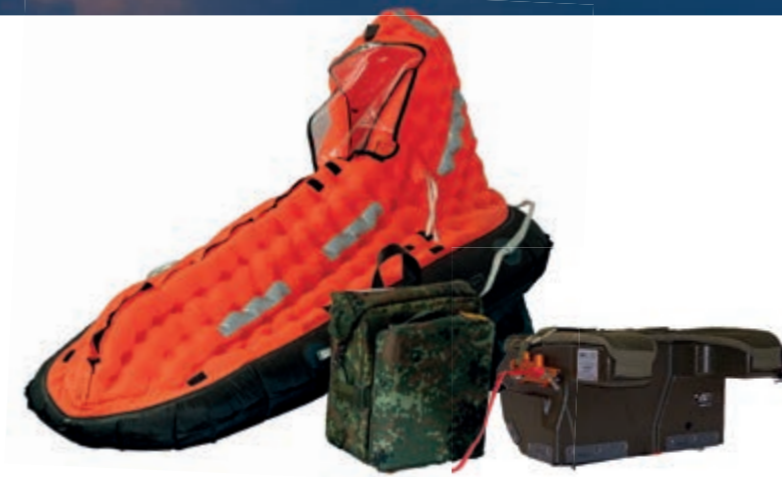
Rescue dinghy and personal survival pack (PSP) as bag and in the seat box version
